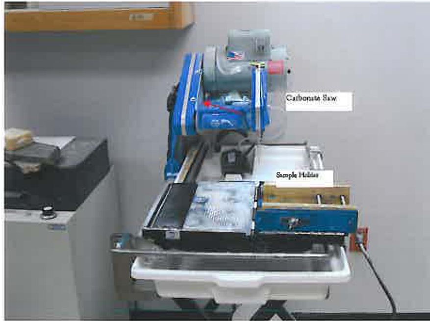
Figure 4: Hydraulic carbonate saw used to slice coral cores into slabs for x-radiograph analysis.
