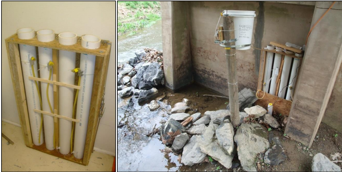
Figure 6: Image of the completed filter columns and their location on Woods Creek in Lexington, VA under a bridge.
