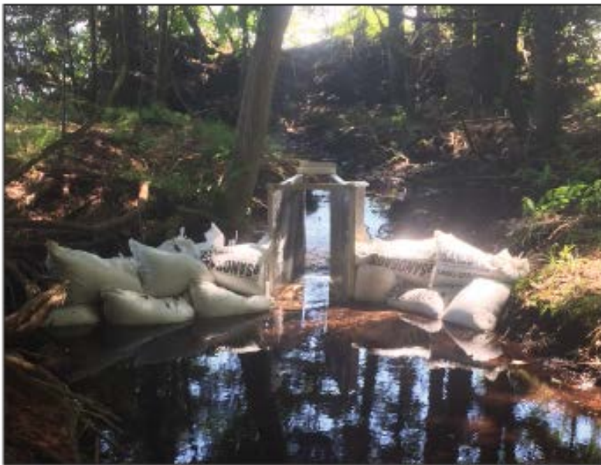
Figure 3: The Parshall flume installed to measure discharge on Honeysuckle Creek. The stream samples were taken just downstream of this flume. The photo was taken downstream and the flume measured a half a foot wide.
