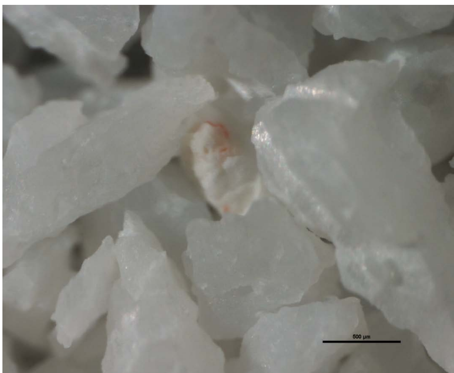
Figure 5 A contaminant settled between pure aragonite fragments being examined beneath the binocular microscope (Sample M8f-BZ-CG-TW15).
