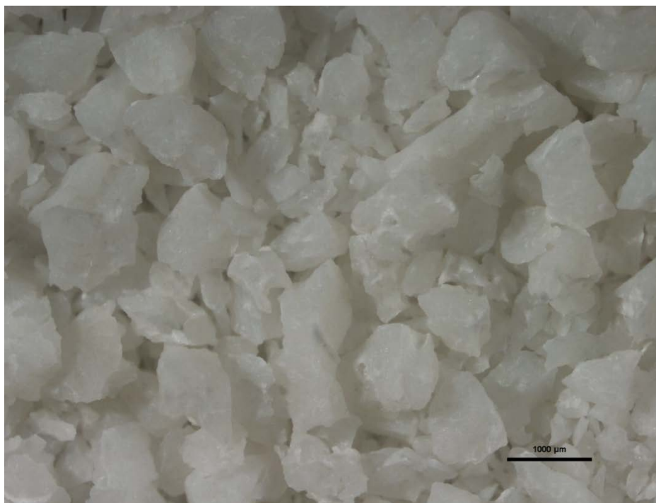
Figure 4 Clean aragonite fragments beneath the binocular microscope (Sample A2a-BZ-CG-TW15).
