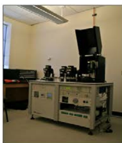
ASI Alphachron for He extraction and measurement
