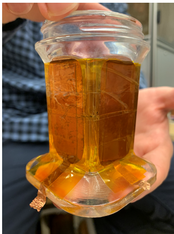
Figure 3.23: Our modified staining jar for the application of electric fields parallel and perpendicular to the surface of a slide during nanoparticle assembly. The capacitor plates are constructed from copper tape. Insulating tape prevents sparking between plates when two fields are applied simultaneously.
