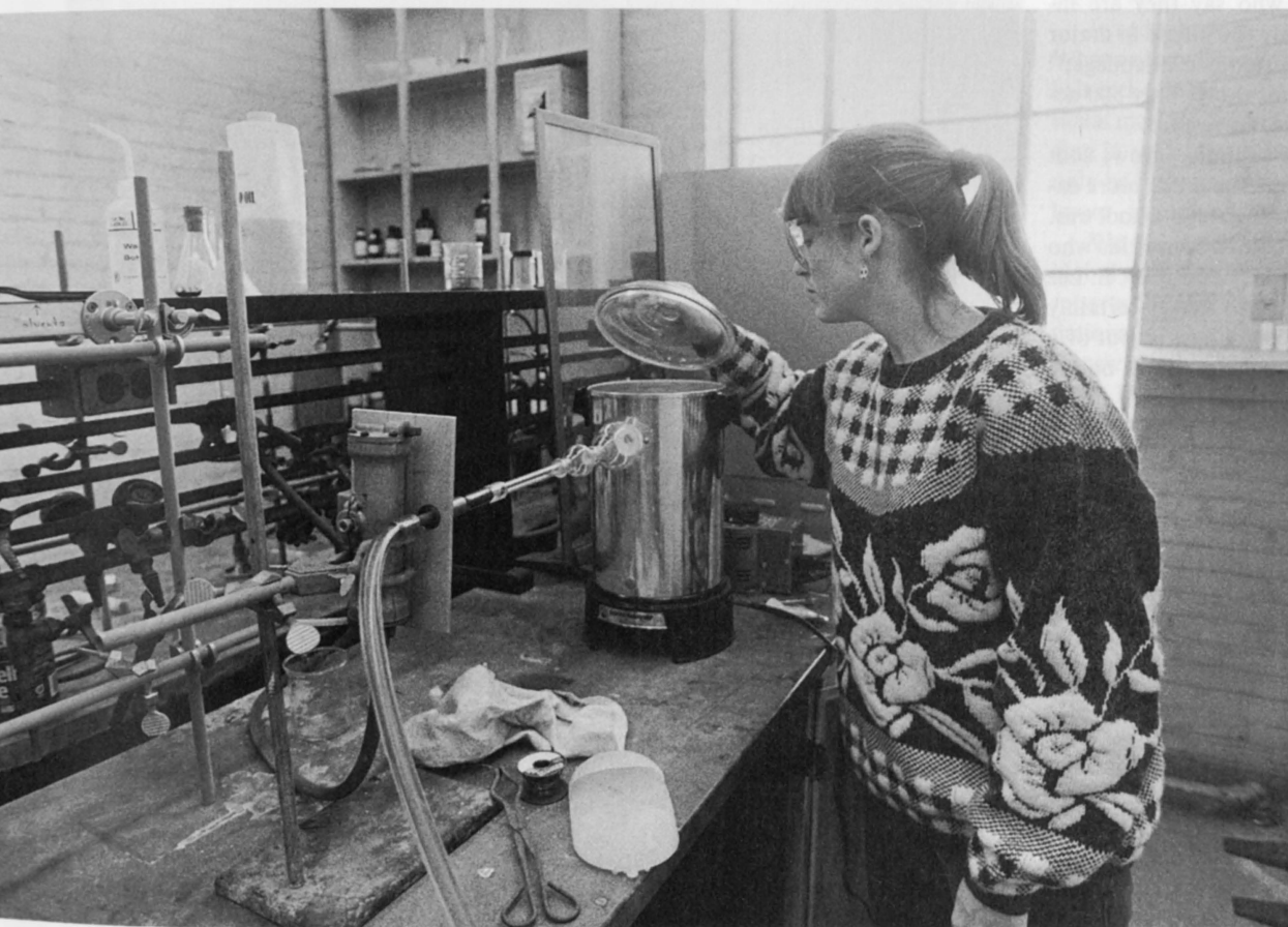
Budding researcher Sarah Allen takes a peek inside her Kugelrohr, a contraption that distills chemical solutions.
