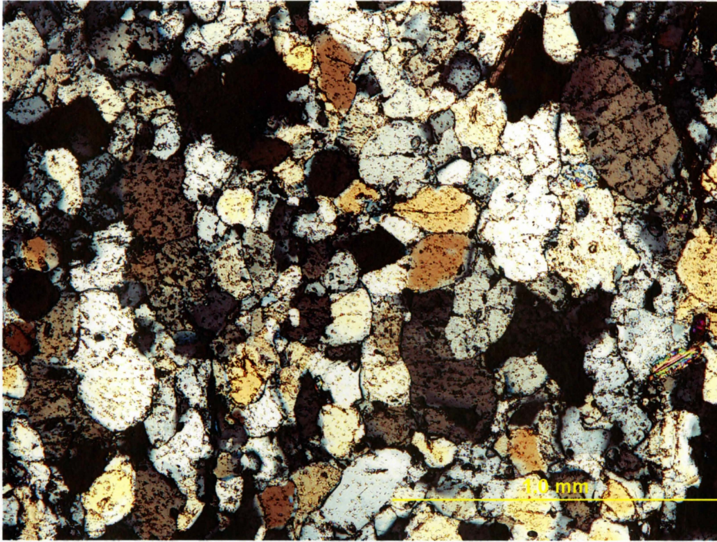
Figure 21: Granoblastic medium grain texture.
