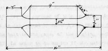
For material from which it is impracticable to obtain test specimens like those for sheared plates, the test specimen may be planed or turned parallel throughout its entire length, and in cases where possible two opposite sides of the test specimen shall be rolled surfaces. Small rolled bars of uniform section shall be tested full size as rolled.
