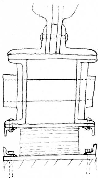
plate. I investigated the plate as a beam and found its thickness in excess of that required. In order to giving bearing area enough for pins two  $1\frac{1}{8}$ " plates must be riveted to the web of the channels as shown.
