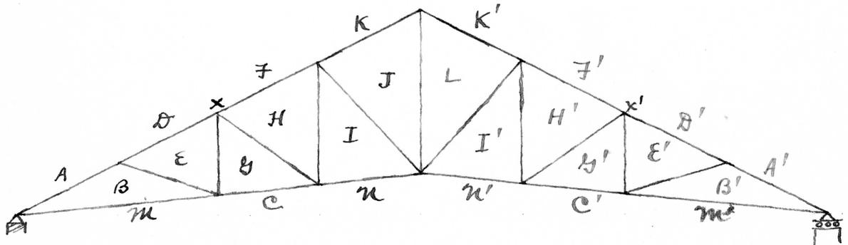
The members  $AB + DE$  and likewise  $A'B' + D'E'$  will be made the same size straight through and also  $FH, KJ, F'H' + K'L$  will be made the same size.
