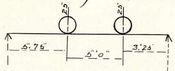
The section of absolute bending moment is as far from the left end as the custer of gravity of the loads is from the right end. Hence the position of the loads is as shown.
