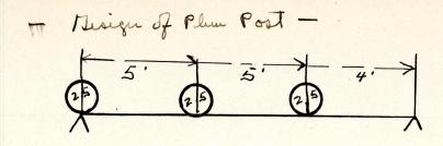
The above loading is for greatest vertical shear in at the support.
