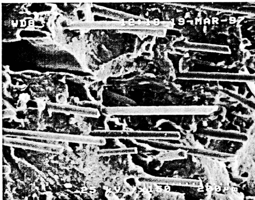
SEM 2- RRTUN - Paralell - Near Surface - Fibers are oriented in a uniform direction near the surface of the material.
