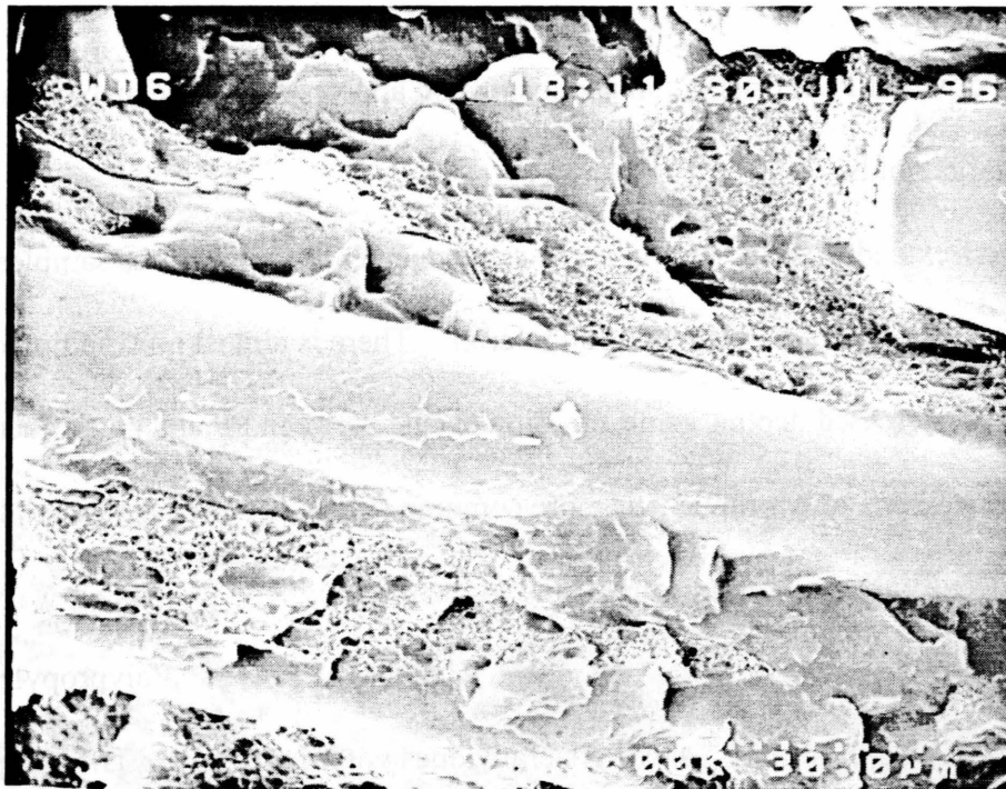
SEM 29 - RRT22 - 6.2 - 12.4 m - The matrix near this fiber shows polypropylene localized about the fiber with PE bordering PP.
