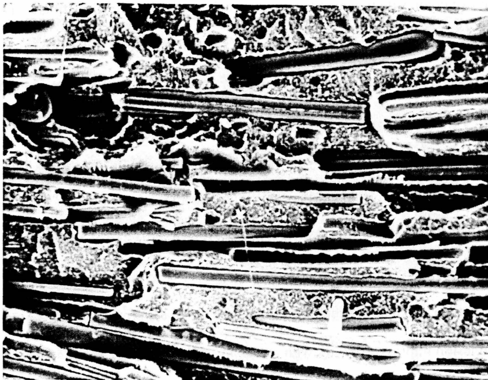
SEM 4 - This figure is a high density polyethylene reinforced with glass fibers (no PP). It is provided for comparison of adhesive qualities
