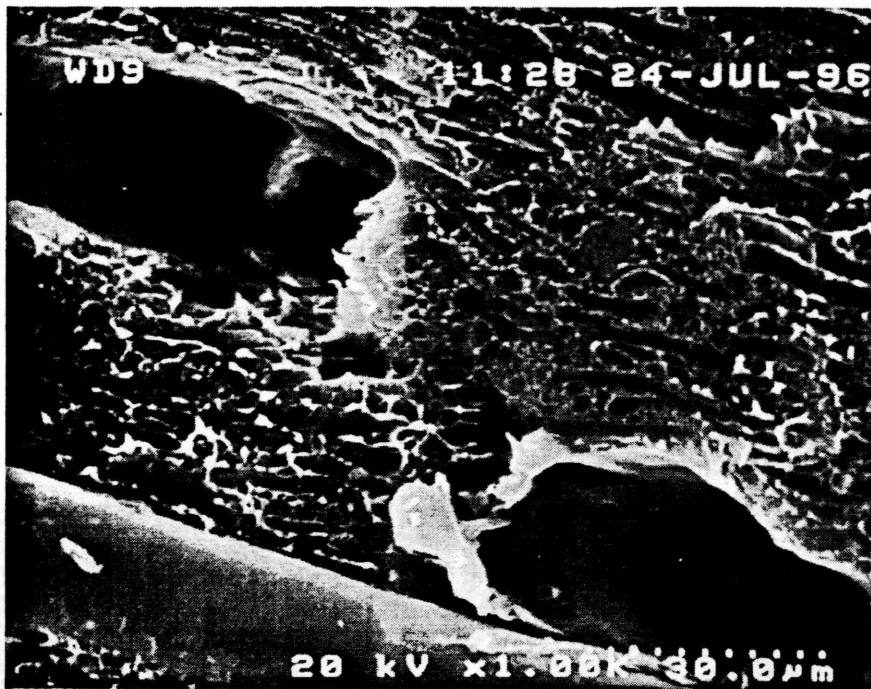
SEM 7 - RRTUN- Parallel- Surface- Holes where glass fibers have pulled out of the matrix. Dispersed phase appears as elliptical streams.
