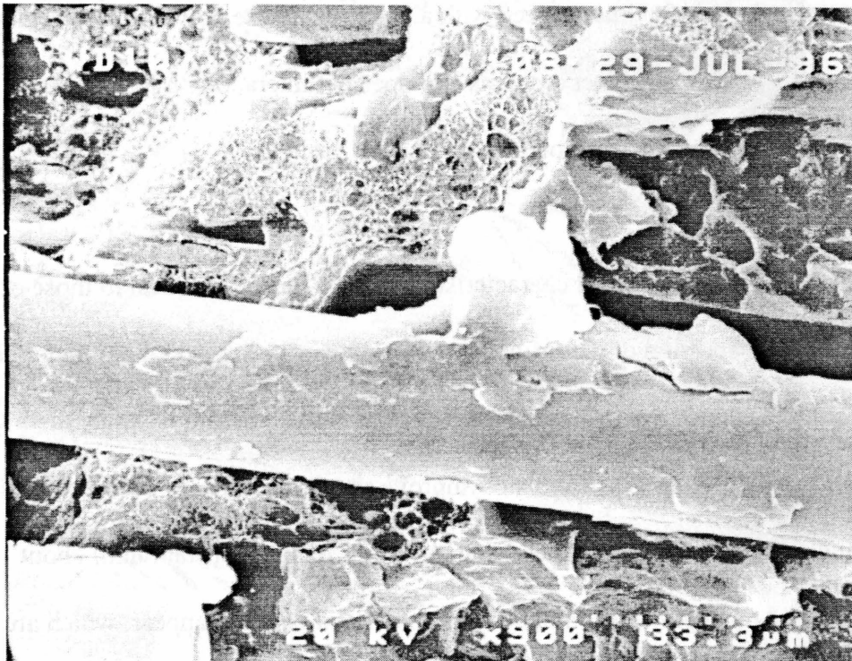
SEM 22 - RRT28 - Parallel - 6.2 - 12.4 mm - There is slight adhesion between Polypropylene and fibers. This adhesion has little effect in strengthening the material
